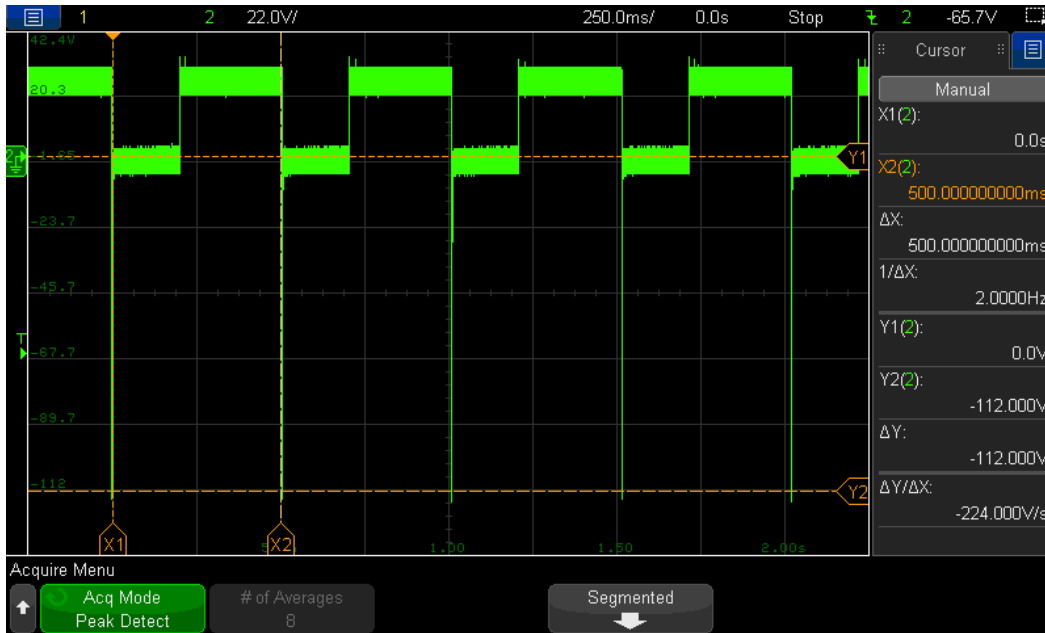
Figure 2.4-3 – Pulse 1 – T1 & T2 – Open Circuit 12 Volts
