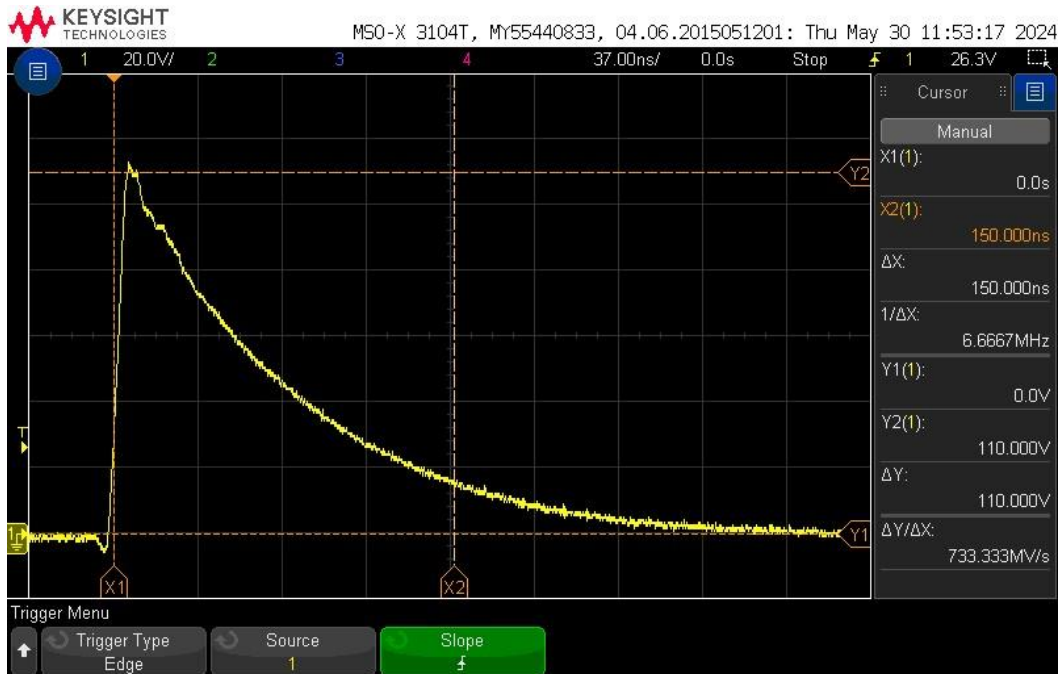
Figure 2.5-2 – Us & Td – Open Circuit – Positive Pulse
