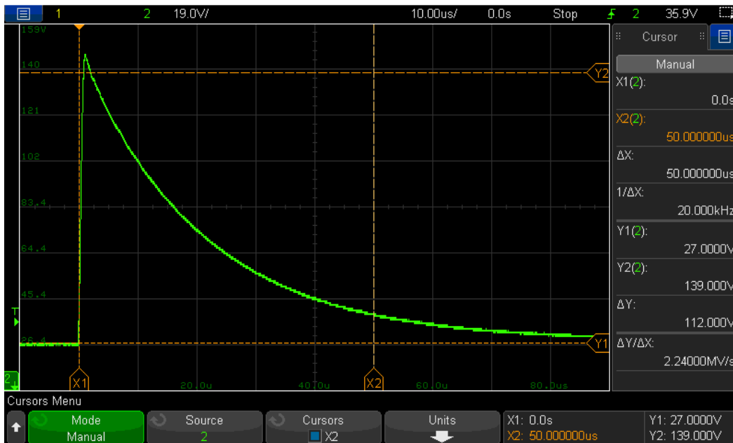
Figure 2.4-17 – Pulse 2a – Td – Open Circuit
