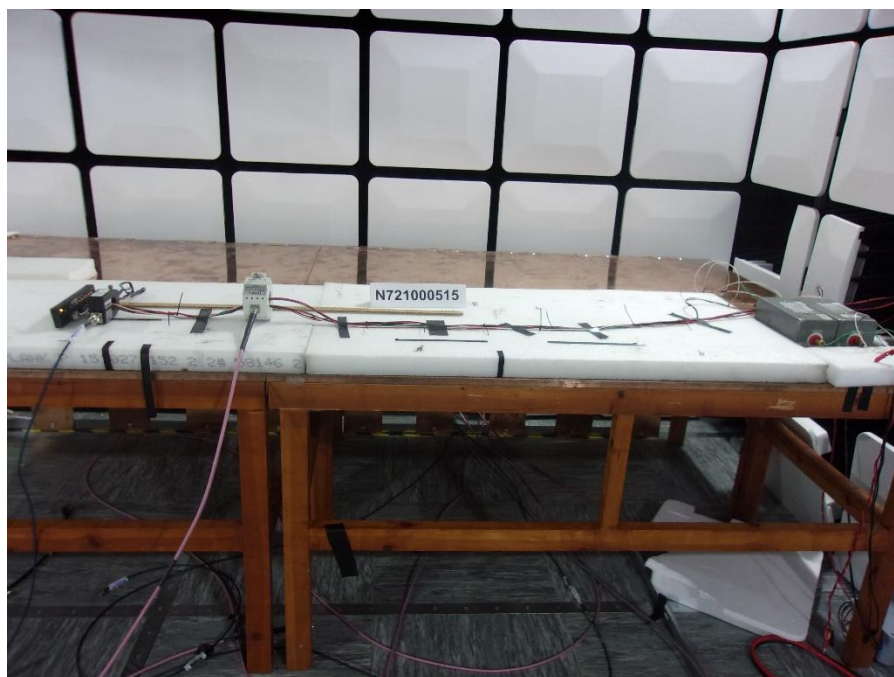
Photo 2.2-2 – ESA RF Immunity Test Setup – BCI 45 CM
