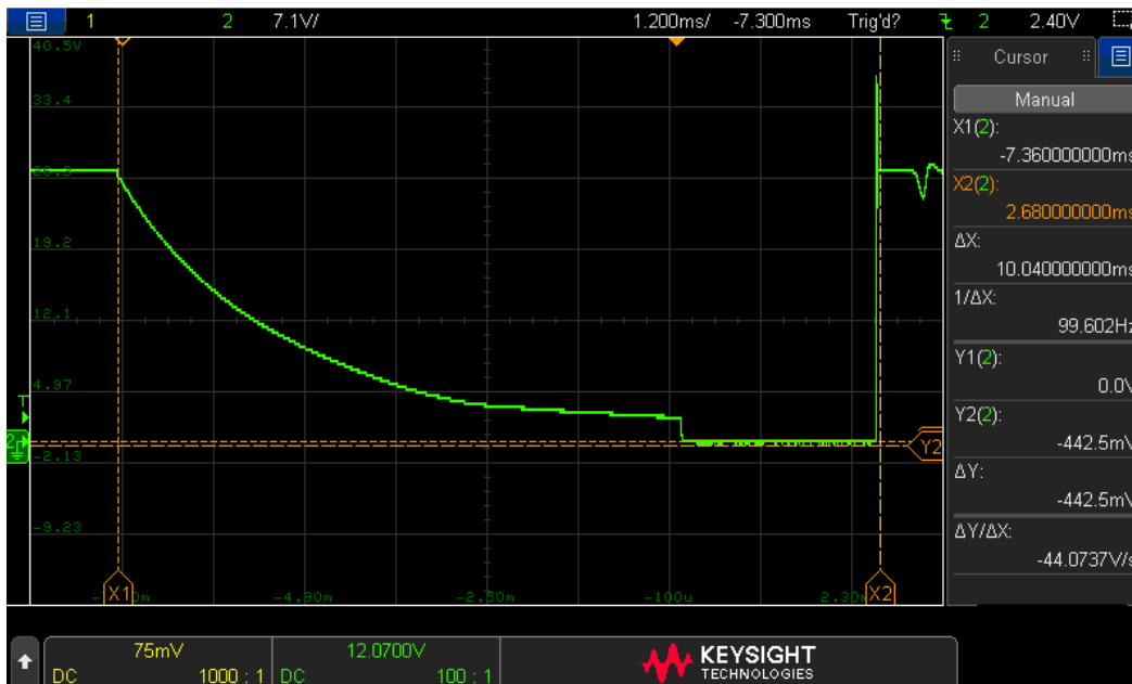
Figure 2.7-2 – Input Power Switched Off – Slow Pulse – Negative
