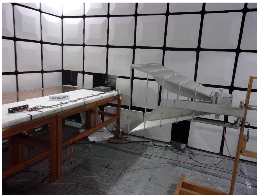
Photo 2.2-4 – ESA RF Immunity Test Setup – Radiated – 200-1000 MHz
