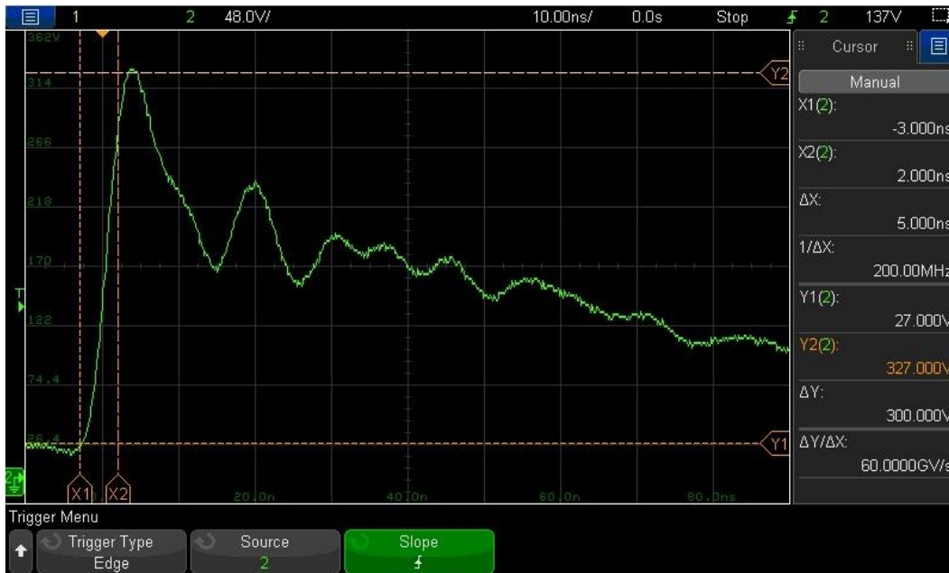
Figure 2.4-32 – Pulse 3b – Us & Tr – Open Circuit
