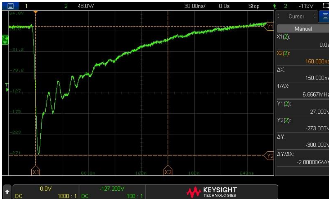
Figure 2.4-25 – Pulse 3a – Us & Td – Open Circuit
