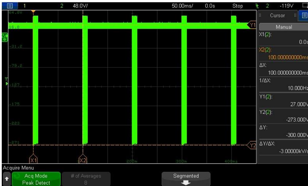
Figure 2.4-27 – Pulse 3a – T4 & T5 – Open Circuit
