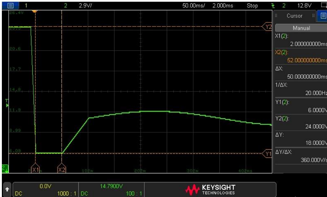
Figure 2.4-46 – Starting Profile – Us, Us6, & T6 – Open Circuit Level III
