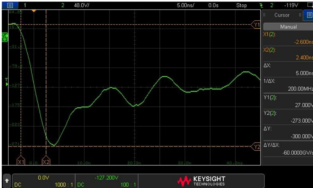
Figure 2.4-24 – Pulse 3a – Us & Tr – Open Circuit
