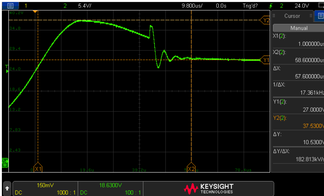
Figure 2.7-3 – Input Power Switched On – Slow Pulse
