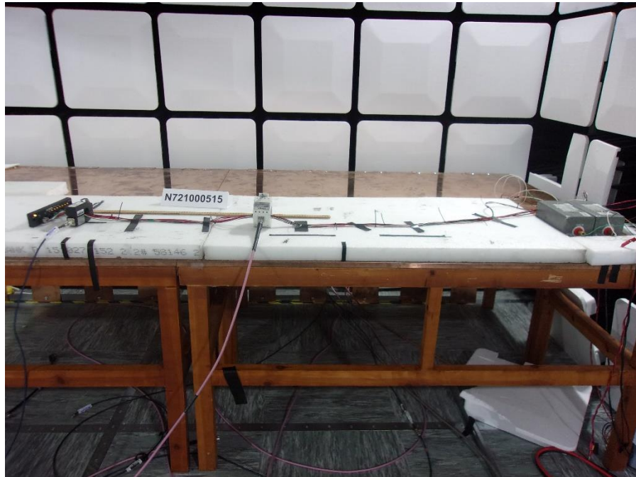
Photo 2.2-3 – ESA RF Immunity Test Setup – BCI 75 CM
