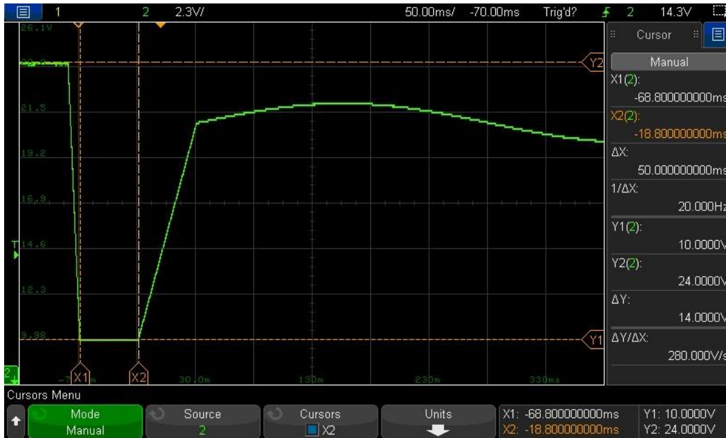
Figure 2.4-40 – Starting Profile – Us, Us6, & T6 – Open Circuit Level I
