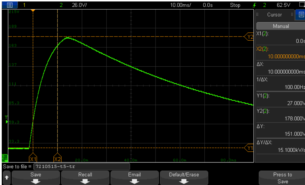
Figure 2.4-49 – Pulse 5a – Tr & Us – Open Circuit
