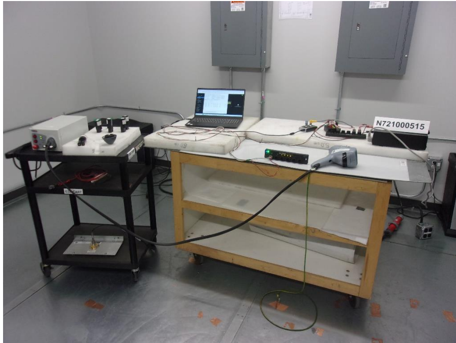
Photo 2.3-1 – ESD Test Setup Photo
