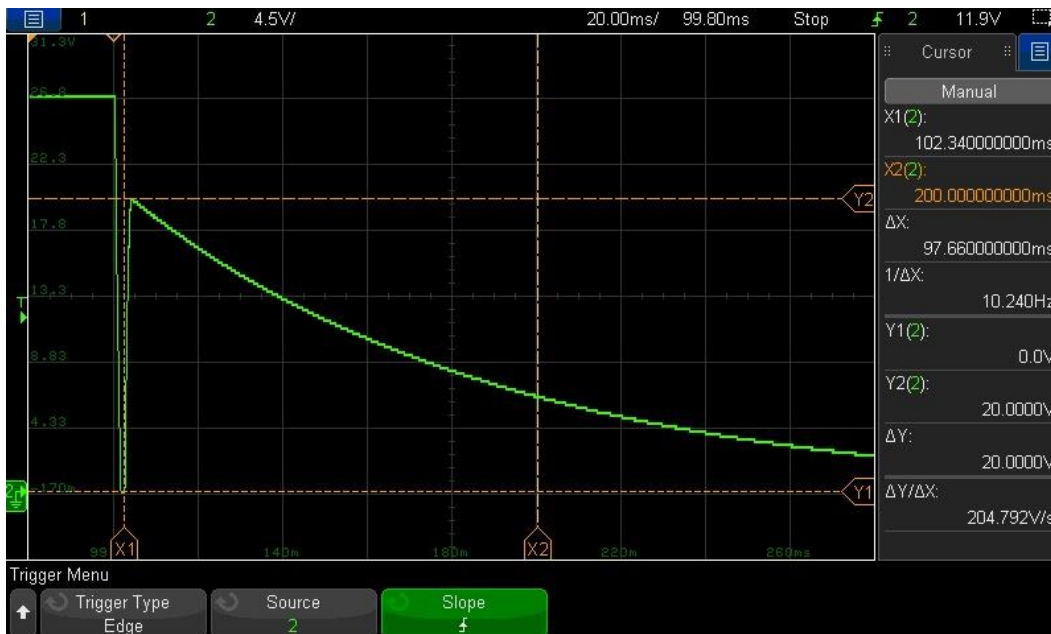
Figure 2.4-22 – Pulse 2b – Td – Open Circuit
