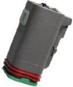
4 Pin CAN Terminating Plug DP-34042-402 120 Ohm terminating resistor on pin 2 and pin 4.
