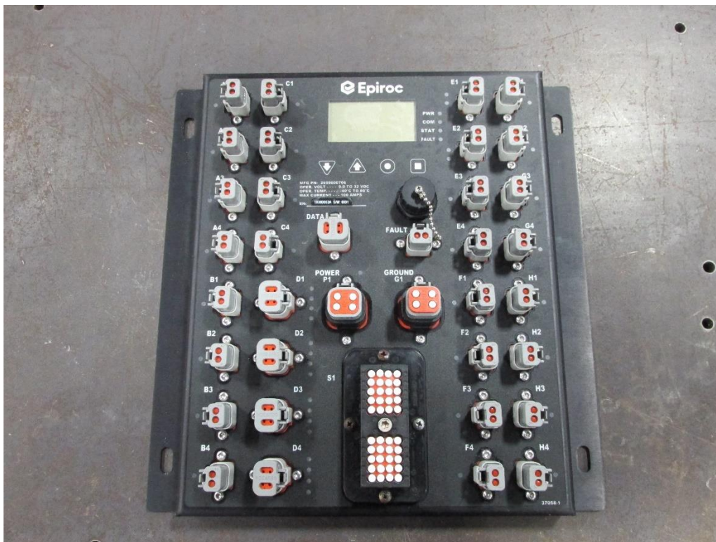
Figure A58: Sample 53A Post-Soak 50/50 Green Antifreeze (Front)
