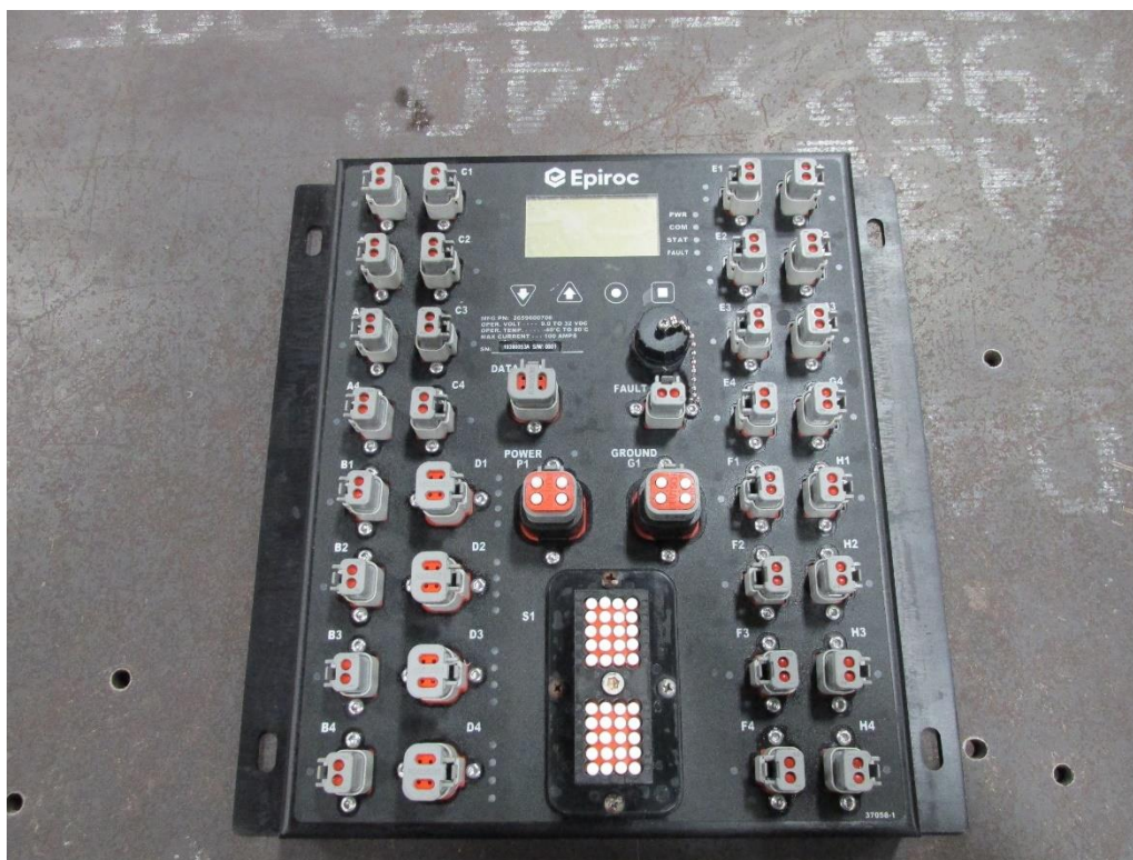
Figure A38: Sample 53A Post-Soak Calcium Hydroxide (Front)
