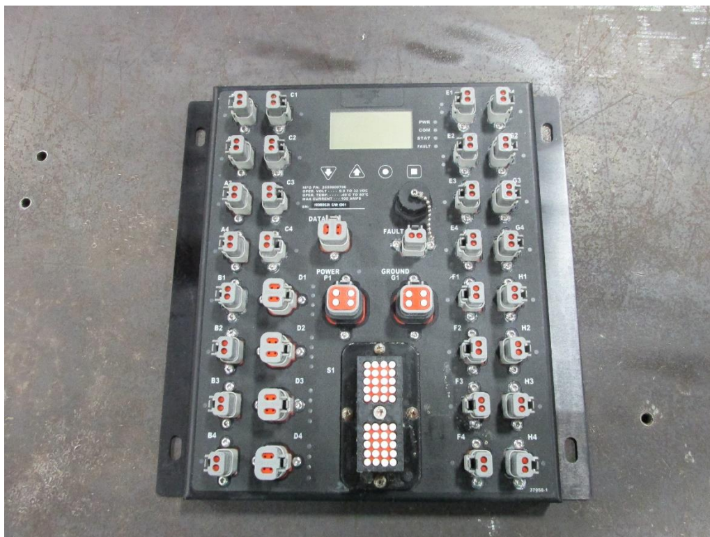
Figure A21: Sample 52A Post-Soak Diesel Coated (Front)
