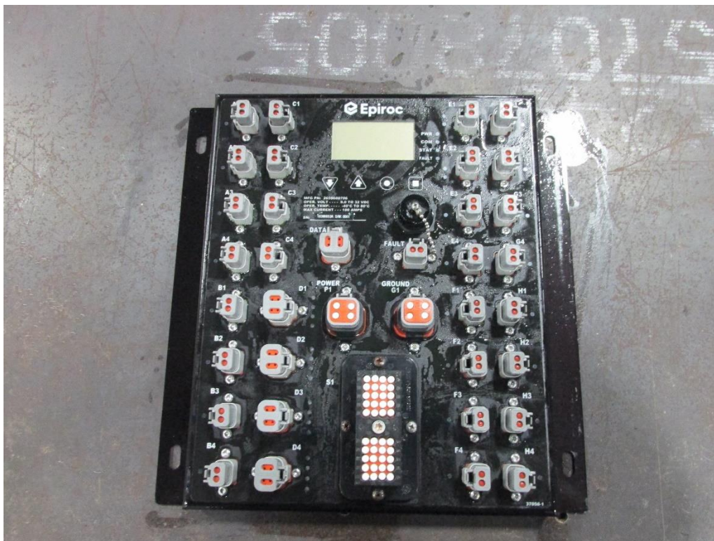
Figure A56: Sample 53A Pre-Soak 50/50 Green Antifreeze (Front)
