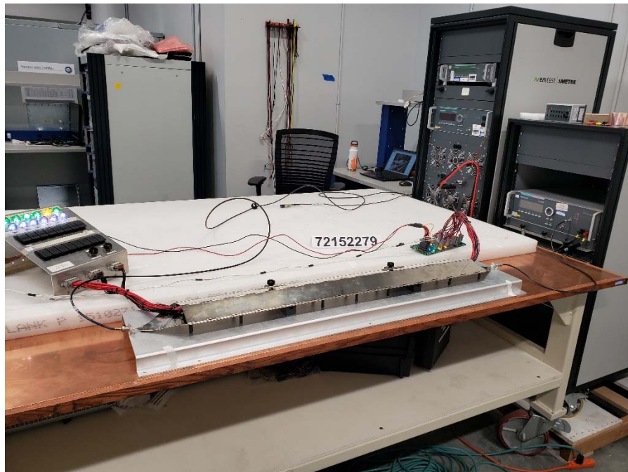
Photo 2.3.8-2 – Immunity to Conducted Transients [CCC Method]
