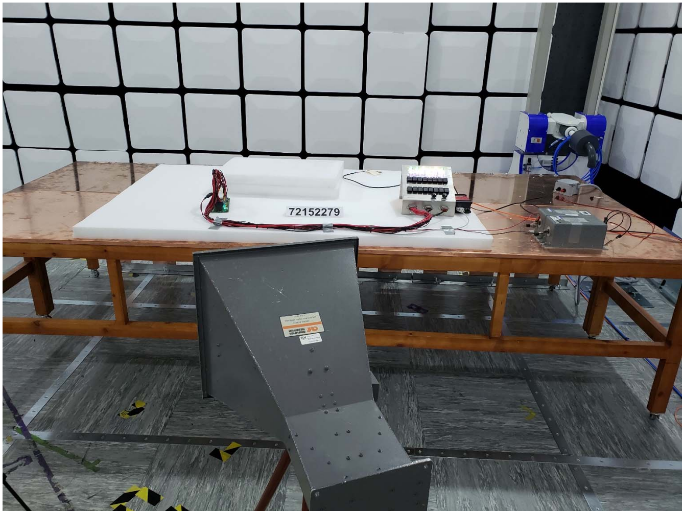
Photo 2.5.6-2 – Electromagnetic Field Immunity Test Set-up – 1000-2700MHz
