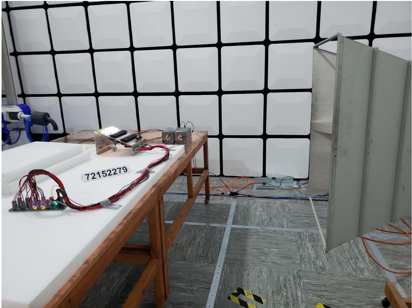
Photo 2.5.6-1 – Electromagnetic Field Immunity Test Set-up – 400-1000MHz
